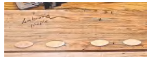
▲ Pic.7 For the box bottom I took two pieces of 180 × 180 × 20mm Ambrosia maple boards and glued them together using four No.20 biscuits
